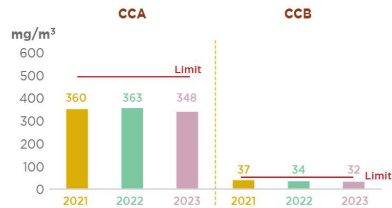
Atmospheric NO x emissions levels in Coloane Power Station
